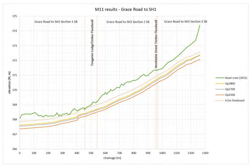
Figure 10 MIKE11 modelled water levels for various discharges compared against right bank flood protection scheme assets between Grace Road and SH1.
