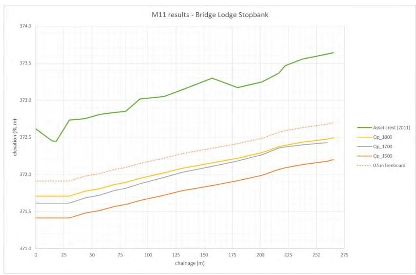
Figure 11 MIKE11 modelled water levels for various discharges compared against the left bank flood protection scheme asset Bridge Lodge Stopbank.
