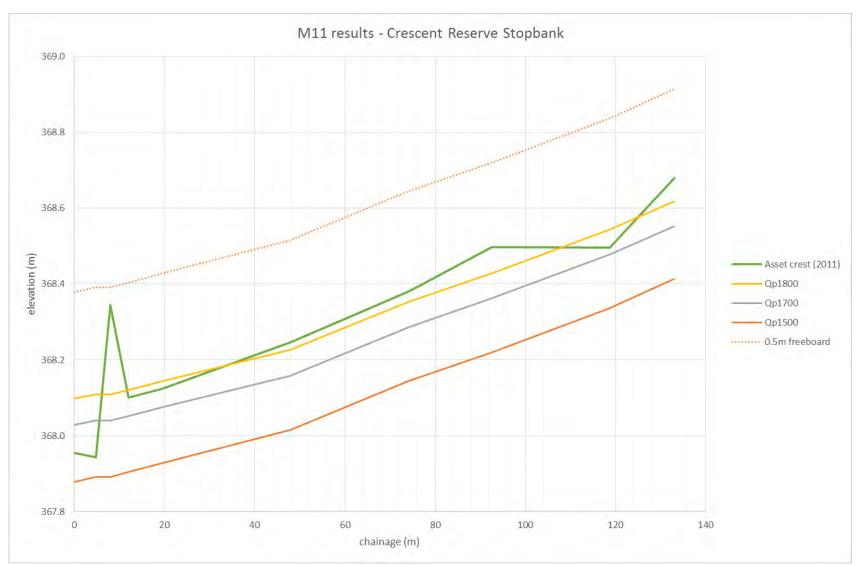
Figure 12 MIKE11 modelled water levels for various discharges compared against the left bank flood protection scheme asset Crescent Reserve Stopbank.
